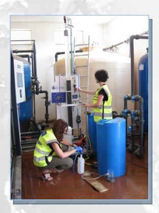
Different tests have been carried out with the labscale pilot plant in situ at the **Benizalon** DWTP. This experimentation has been carried out as a preliminary stage to the construction of the pilot plants in Almeria, for the **optimization** of some of the operation parameters and to evaluate the efficiency of the filtering materials.
