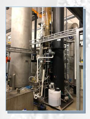
The pilot plant is already **installed** and **running** at the **Viimsi** DWTP (Estonia). The design of this plant has been focused on **removing Ra-226**, **Ra-228**, besides other water pollutants.
