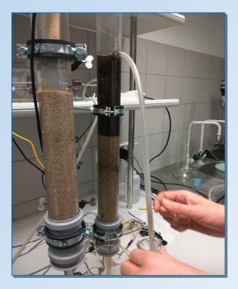
Lab scale studies with the hydrous manganese oxide (HMO) process were carried out to remove iron, manganese and radionuclides from water, and several different combinations of filter materials like dolomite, anthracite, zeolite, sand and gravel were tested.
