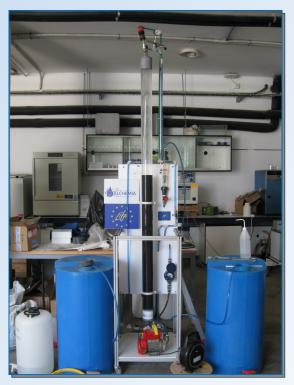
CIESOL proceeded to the construction of a lab-scaled pilot plant. The plant will allow checking the granular materials available on the market to achieve the removal of the radionuclides contained in the water according to different strategies.
