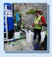
In order to verify the compliance with the drinking water quality standards and the optimal operation of the pilot plants, the CIESOL team has carried out the first sampling in the filtration, washing and filter material stages of the filtration tanks.
