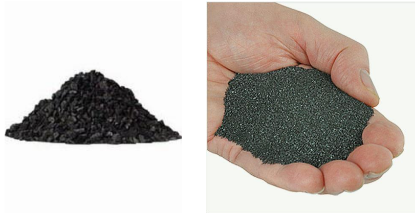
Figure 5. Granular MnO 2 and GreensandPlus ™
